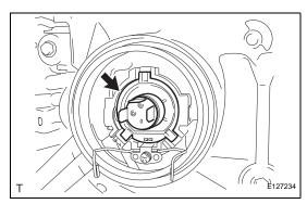
(c) Remove the headlight, No. 1 bulb.NOTICE:Do not touch the bulb glass with your fingers.
